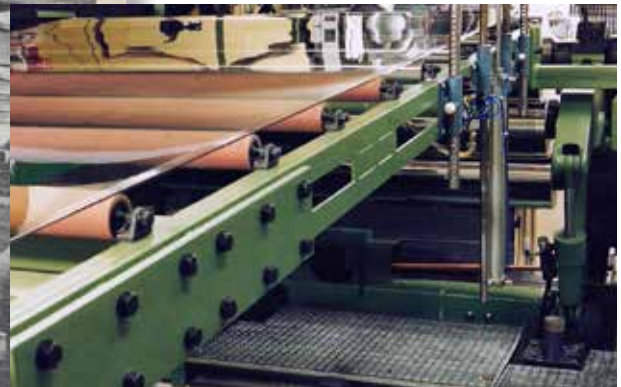
The Reifenhäuser, the first extruder designed exclusively for polycarbonate and able to produce sheets two metres wide.
